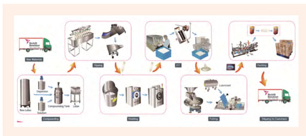
Figure 3. RB Condom production process
